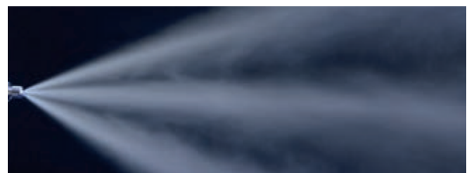
Spray pattern of a flat fan nozzle
