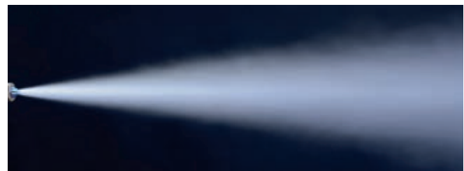
Spray pattern of a Laval nozzle
