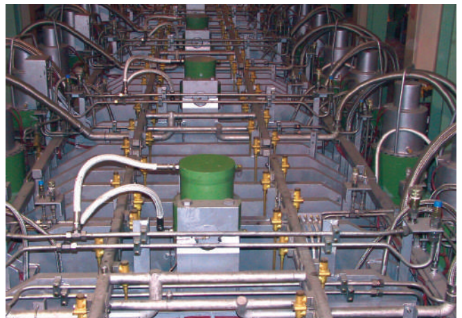
Horizontal segments with Mastercooler SMART nozzles
